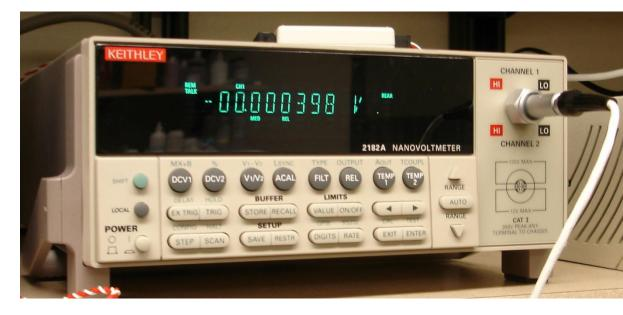
The two-channel Model 2182A Nanovoltmeter is optimized for making stable, low noise voltage measurements and for characterizing low resistance materials and devices reliably. It provides higher measurement speed and significantly better noise performance than alternative low voltage measurement solutions. It offers a simplified delta mode for making resistance measurements in combination with a reversing current source, such as the Model 6220 or 6221.
