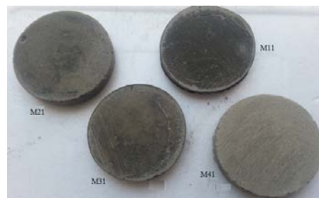
Figure 3b: High compressive strength Polished geopolymer inorganic membrane
