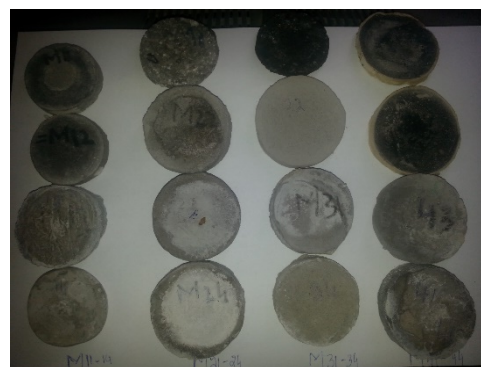
Figure 3a: Hydrothermal treated geopolymer membranes
