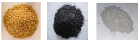
Figure 2: (a) Rice Husk (RH) (b) Rice husk Ash (c) Thermally treated (RHA)
