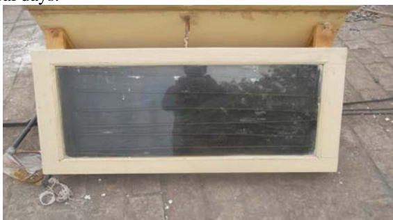
Fig. 1. Photograph of flat plate solar collector
