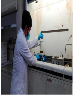
Fume hoods are generally set back against the walls and are often fitted with infills above, to cover up the exhaust ductwork. Because of their shape they are generally dim inside, so many have internal lights with vapor-proof covers. For exceptionally hazardous materials, an enclosed glove box may be used, which completely isolates the operator from all contact with the work material and tools.
