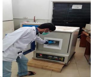
Max temperature:1800°C, Chamber size: 150\*150\*150mm, 200\*200 zoomm, 300 500 500 mm, realing element. WOOZ neater, Chameber Size:200\*200\*200mm (8\*8\*8inch), Max. temperature:1800°C, Work temperature:1700°C, Temperature control:30segments programable and PID auto control, Heating elements: MoSi<sub>2</sub> heater, Thermocouple: B type, Heating rate:0-40C/min, Temperature accuracy:+/-1C, Power: AC208-240V, 50/60HZ, Single phase, Max power:8KW, Net weight:170kgs
