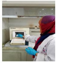
A muffle furnace is a furnace with an externally heated chamber, the walls of which radiantly heat the contents of the chamber, so that the material being heated has no contact with the flame. Muffle furnaces are most often utilized in laboratories as a compact means of creating extremely high-temperature atmospheres. They are employed to test the characteristics of materials at extremely high and accurate temperatures. A muffle furnace is also known as a retort furnace.
