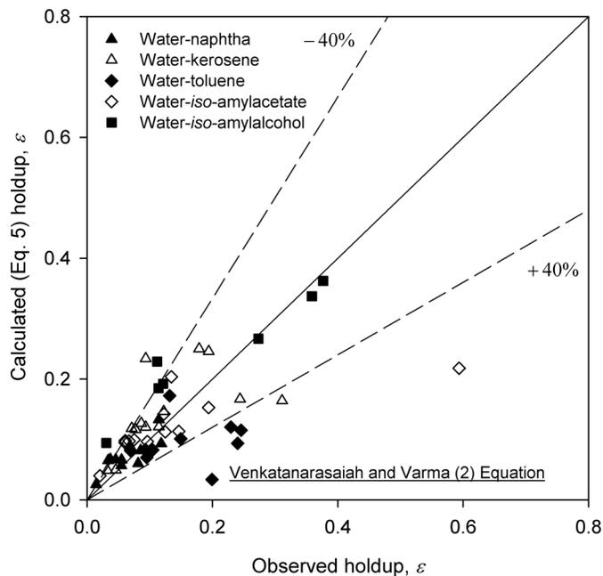
FIG. 8. Scatter diagram between observed holdup and holdup calculated from Eq. (4).
