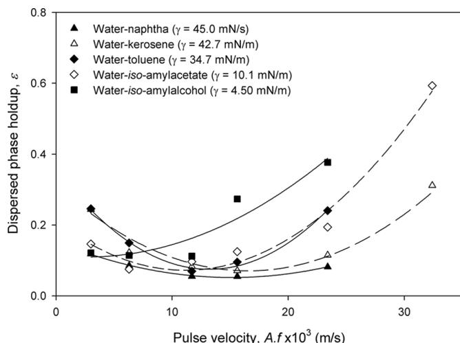
FIG. 2. Effect of pulse velocity on the dispersed phase holdup without mass transfer.  $u_d = 2.73 \times 10^{-3}$  m/s,  $u_c = 2.86 \times 10^{-3}$  m/s. For naphtha:  $u_d = 2.47 \times 10^{-3}$  m/s. The data for water-kerosene and water-iso-amylacetate is taken from Khawaja et al. (21).
