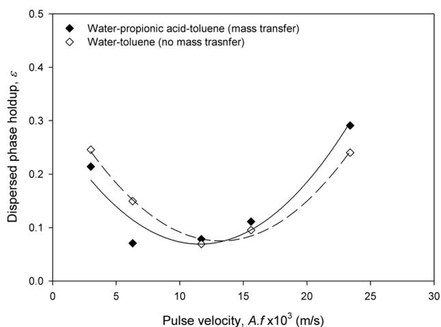
FIG. 4. Comparison of the effect of pulse velocity on the dispersed phase holdup with and without mass transfer for water-propionic acid-toluene.  $u_d = 2.73 \times 10^{-3}$  m/s,  $u_c = 2.86 \times 10^{-3}$  m/s.
