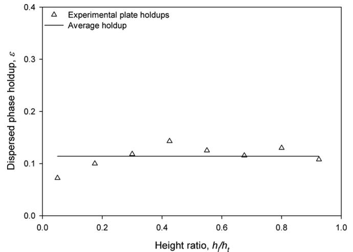
FIG. 1. Variation of dispersed phase holdup with height ratio (defined as height of the *i*th sampling point from the bottom of the column to the total effective column height) and average of these holdups for the *iso*-amylalcohol-water system.  $A \cdot f = 6.3 \times 10^{-3}$  m/s,  $u_d = 2.73 \times 10^{-3}$  m/s,  $u_c = 2.86 \times 10^{-3}$  m/s.
