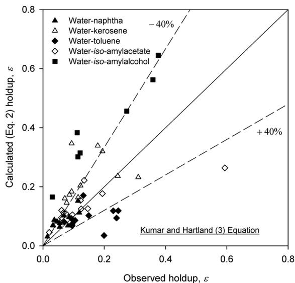
FIG. 7. Scatter diagram between observed dispersed phase holdup and the dispersed phase holdup calculated from Eq. (2).
