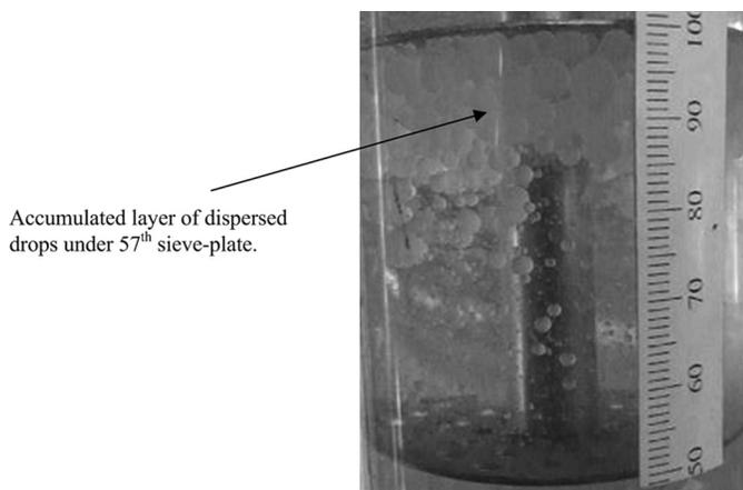
FIG. 3. Mixer-settler region showing accumulation of dispersed phase (toluene) drops under 57th sieve-plate for the water-toluene system.  $A \cdot f = 6.3 \times 10^{-3}$  m/s,  $u_d = 2.73 \times 10^{-3}$  m/s,  $u_c = 2.86 \times 10^{-3}$  m/s.
