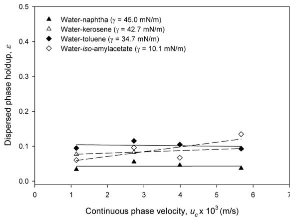
FIG. 5. Effect of continuous phase superficial velocity on the dispersed phase holdup.  $A \cdot f = 11.7 \times 10^{-3}$  m/s,  $u_d = 2.73 \times 10^{-3}$  m/s. For naphtha:  $u_d = 2.47 \times 10^{-3}$  m/s. The data for water-kerosene and water-*iso*-amylacetate is taken from Khawaja et al. (21).
