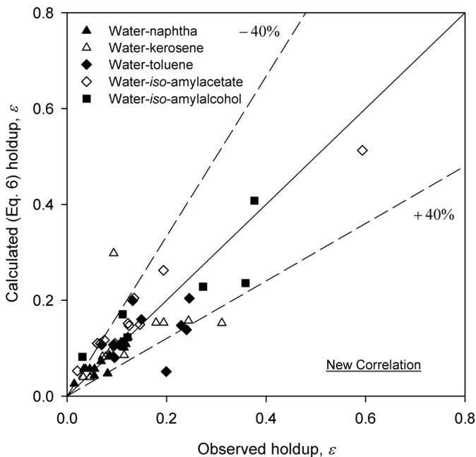
FIG. 9. Scatter diagram between observed holdup and holdup calculated from the new development correlation Eq. 5.
