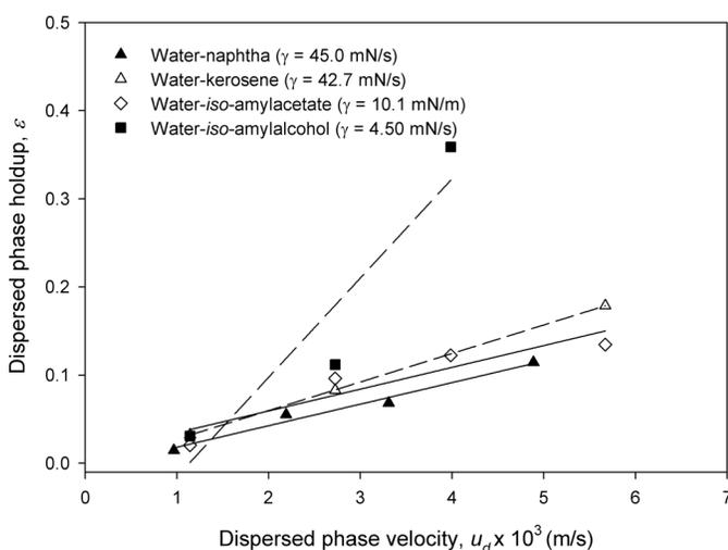
FIG. 6. Effect of dispersed phase superficial velocity on the dispersed phase holdup.  $A \cdot f = 11.7 \times 10^{-3}$  m/s,  $u_c = 2.86 \times 10^{-3}$  m/s. The data for water-kerosene and water-*iso*-amylacetate is taken from Khawaja et al. (21).
