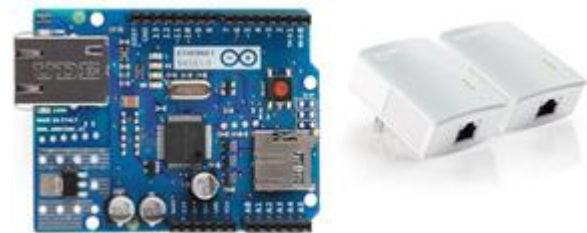
Arduino Ethernet Shield & Power Line Adapter (TP-Link AV500)
