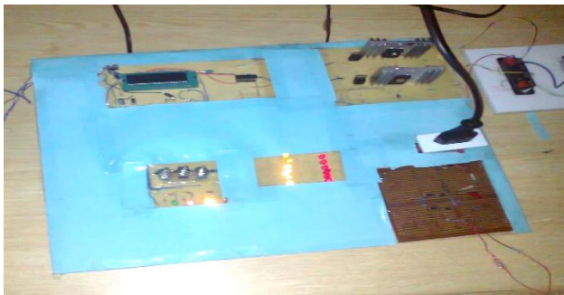
Fig. 4. hardware implementation of Micro-Controller Based PWM inverter
